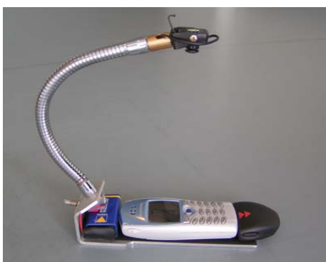
Figure 2. The mini-camera with the mobile barcode scanner system attached.
