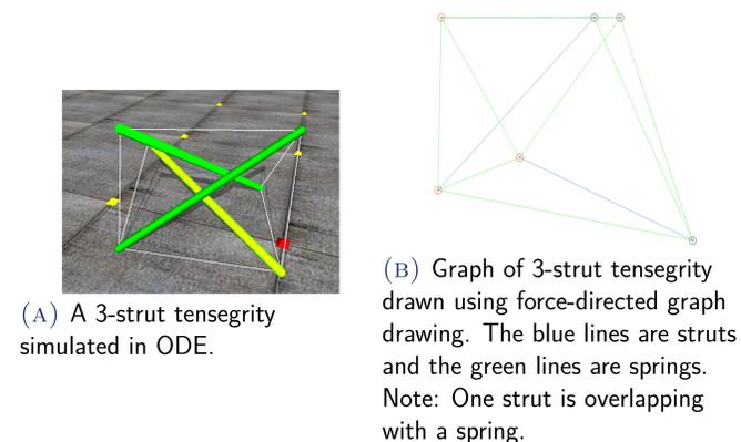
FIGURE 2: Models of the 3-strut tensegrity.
