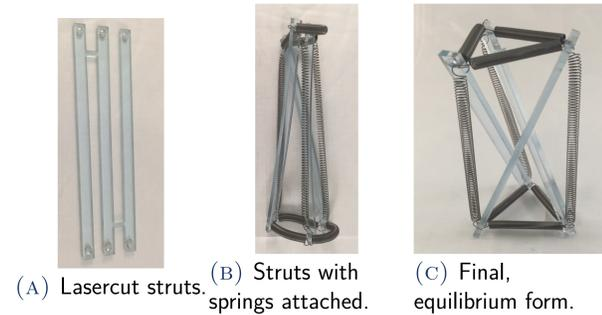
FIGURE 3: Physical construction process.
