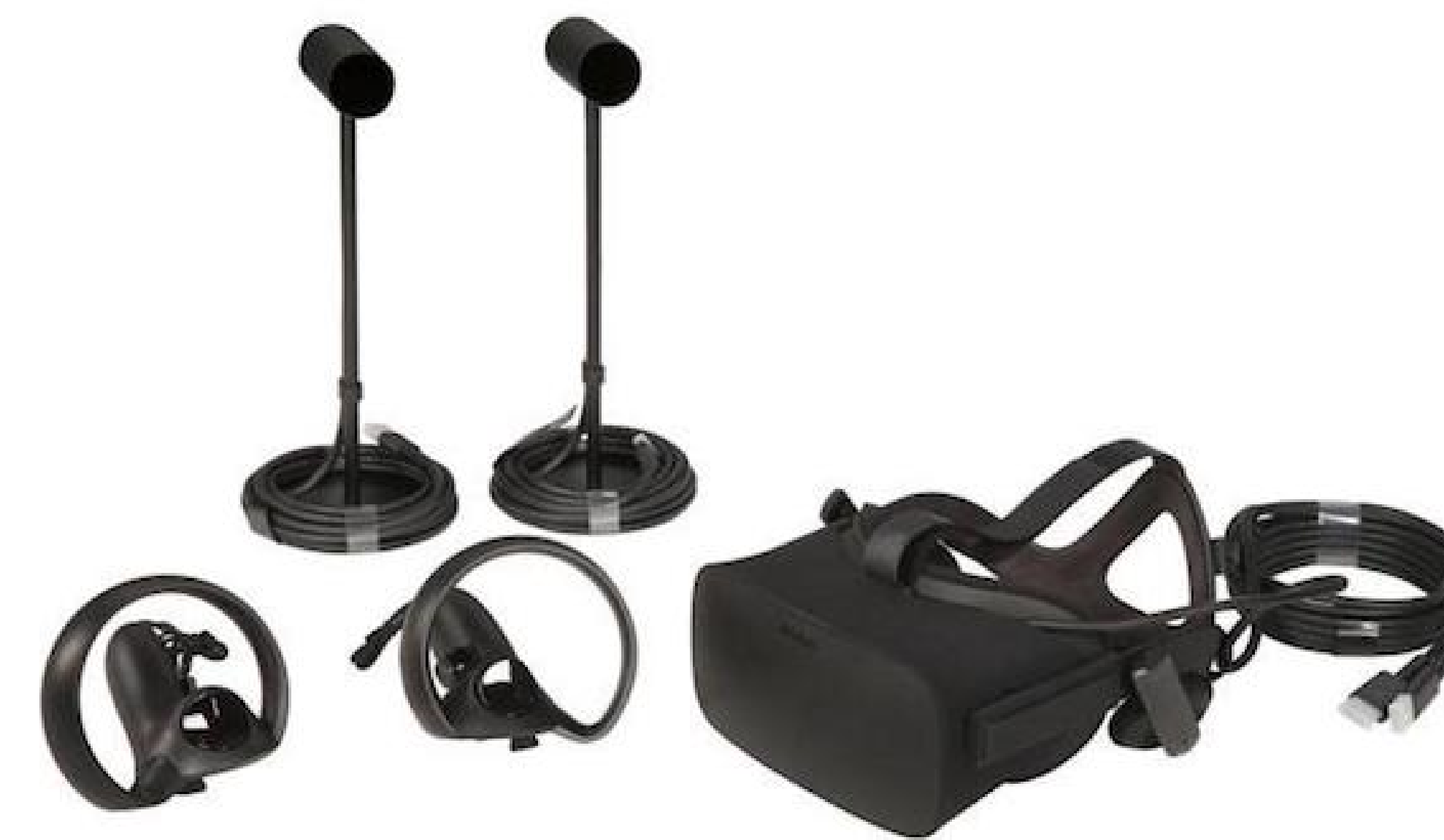
FIGURE 3: Oculus Rift headset, controllers, and sensors
