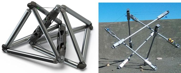
Figure 2: DucTT Robot (Left)<sup>2</sup>; NASA SUPERball Robot (Right)<sup>3</sup>
