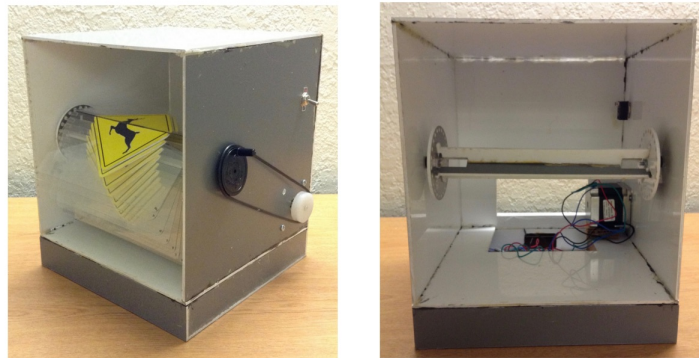
Figure 5: The built Flip Animated Sign
