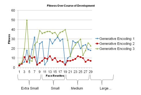
Figure 6: This figure shows the fitness over the course of development for three different generative encodings. Fitness over the course of development can also be referred to as an "ontogenetic trajectory". The robots produced by the encodings are separated into categories of size. Here, each encoding has 10 robots in each category.
