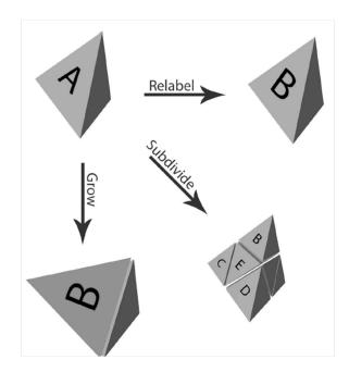
Figure 4: Example rules used in a generative encoding for tetrahedral meshes. Each open face of a tetrahedron is labeled and can have a rule applied to it according to what the generative encoding specifies. The process of evolving a generative encoding modifies the set of rules to produce new designs. Picture from [13].
