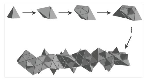
Figure 2: A tetrahedral mesh that is grown using a generative encoding. The robot grows a little larger and more complex each time the rules of the encoding are applied. One application of the ruleset can also be referred to as a "face rewrite". Picture from [13].
