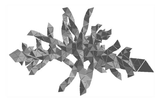
Figure 3: An example of a tetrahedral mesh grown using a generative encoding. Researchers can embed a pager motor into the structure to vibrate it, causing it to move. Picture from [13].
