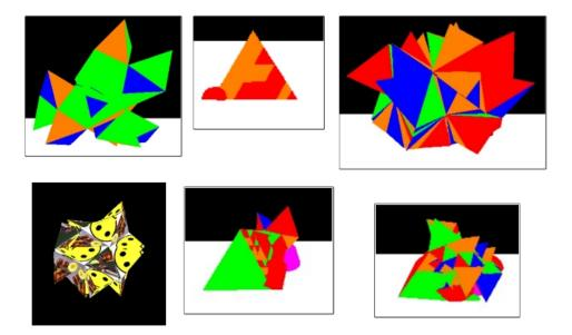
Figure 5: These are some robots that were created and tested in simulation by the genetic algorithm. Each individual is represented by a different generative encoding, each of which is comprised of a different combination of the rules depicted in Figure 4. Every robot is embedded with a vibrational mechanism, represented in the simulation as a pink mass that rotates around a red cylinder. The vibrational mechanism is most clearly visible for the middle robot on the bottom row.
