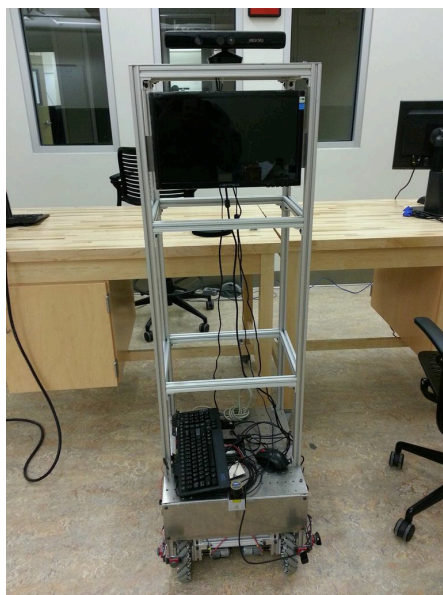
Figure 2: my gesture recognition interface was integrated into Union College's giraffe robot.
